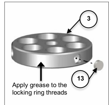
Figure 4-39 Place PTFE Inserts into Adjustment Nut
