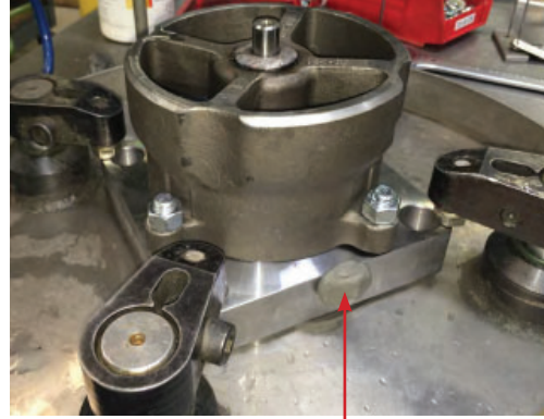
Seal Drain Holes
