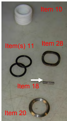
Figure 5-17 Packing, Male Adapter, Spring and O-rings 5.1.9 The seat very critical and must be examined carefully. The crown
