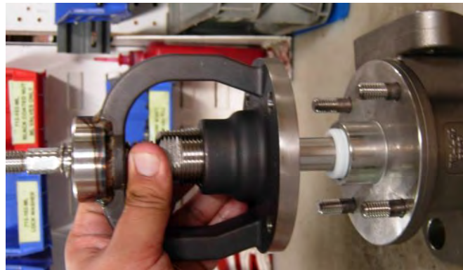
Figure 5-12 Lift Bonnet from Body
