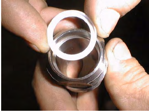
Figure 8-5 Inspect Packing Screw and Wiper
