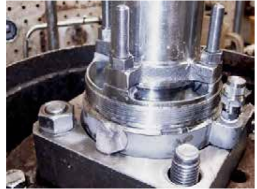
Figure 7-1 Blocking Water Drainage with Putty
