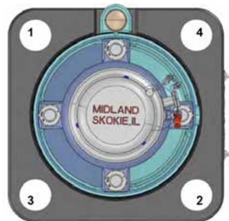
Figure 2-3 Mounting-Nut Tightening Sequence
