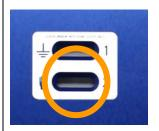
Place the Red Bypass Key over Bypass Window 2 until the green LED lights appear indicating that it is permissible to fill
