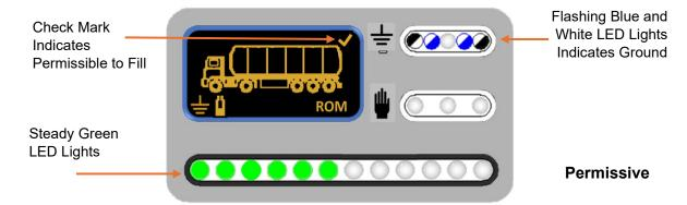
After approximately 15 seconds of inactivity, the truck graphic will change to a timer that is tracking the time the truck has been connected to the monitor (this also prevents the truck graphic from being "burned" into the display). Note: The check mark in the upper right indicates that the truck is permissible to fill.
