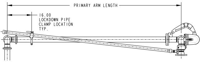
**Note:** Primary Arm Length is the distance between the swivel centerline and the drop-tube centerline. Lockdown clamp is located 16" from the drop-tube centerline.
