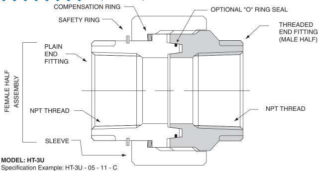
(1/2" UNION Both Ends NPT Threads, Carbon Steel)
