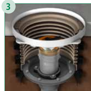
Replace Bellows, Reinstall Upper and Lower Rings
