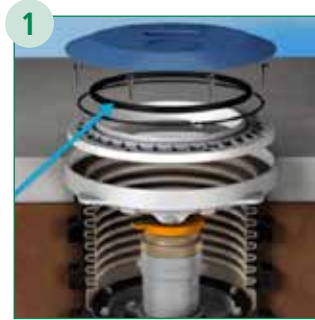
Remove Upper Bolts and Ring
