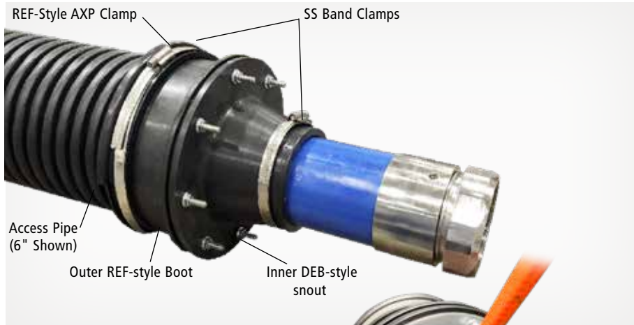
HEF-4020G Entry Fitting with Heat Tracing
