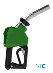
**14C Diesel Capture Technology** – Spout with patented diesel-capture technology. A specially designed chamber inside the nozzle safely captures diesel fuel outside the spout when the nozzle is returned to the cradle. The unique diesel-capture chamber allows the nozzle venturi to evacuate captured diesel fuel from the chamber and reintroduce it into the fuel stream. It's safe, durable and easy to use. The 14C is cULus-listed.
