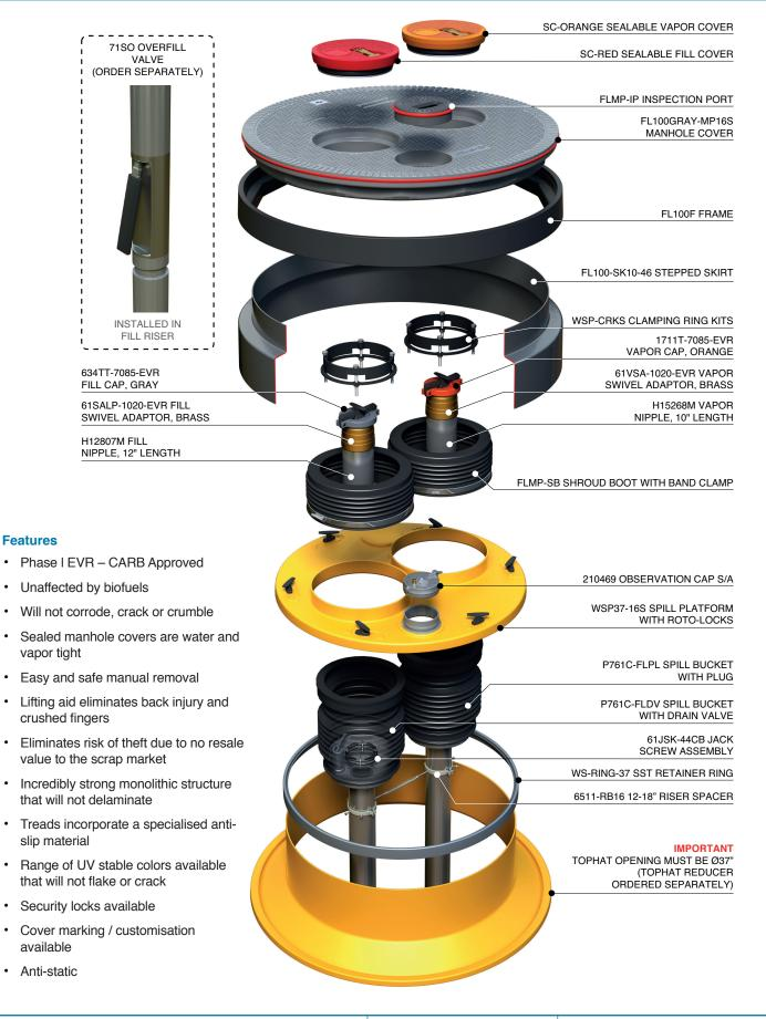
FibreTite multiport kit includes watertight platform for (2) 5-gallon spill buckets, 40" diameter multiport cover, port covers, frame and skirt.
