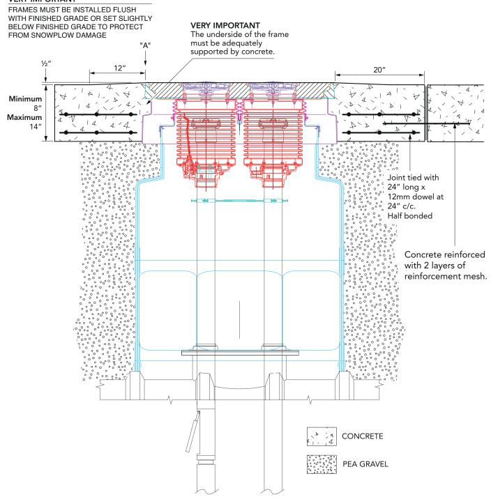
FibreTite multiport kit includes watertight platform for (2) 5-gallon spill buckets, 40" diameter multiport cover, port covers, frame and skirt.
