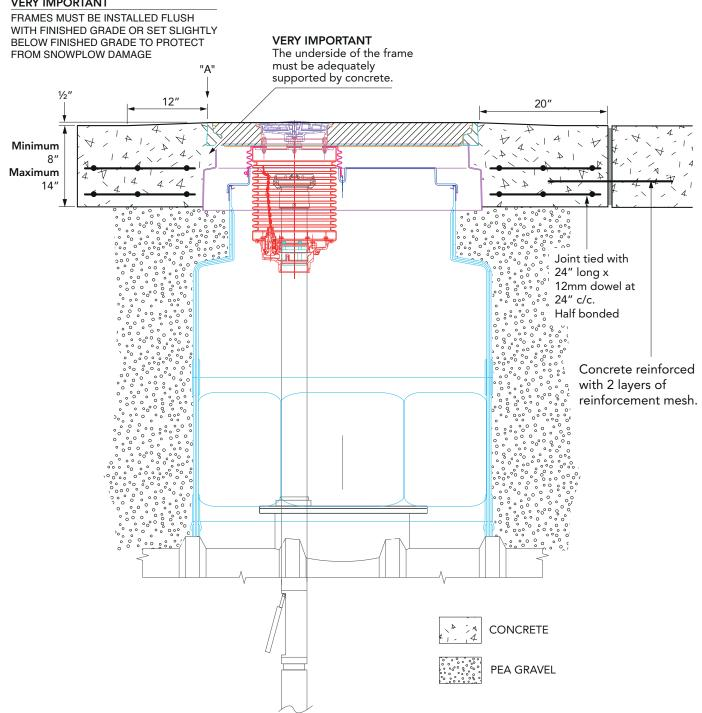
FibreTite multiport kit includes watertight platform for (1) 5-gallon spill bucket, 40" diameter offset cover, port cover, frame and skirt.
