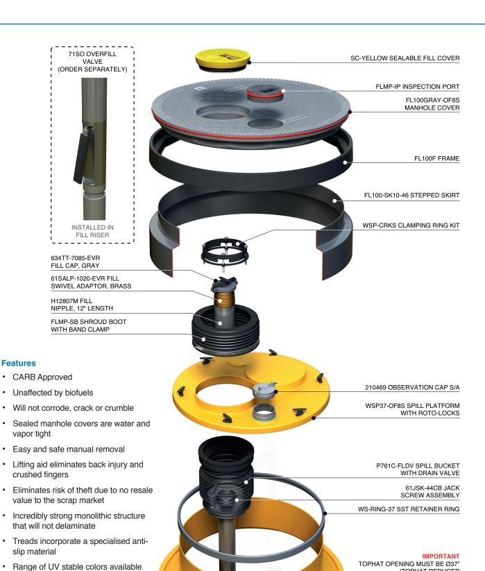
FibreTite multiport kit includes watertight platform for (1) 5-gallon spill bucket, 40" diameter offset cover, port cover, frame and skirt.
